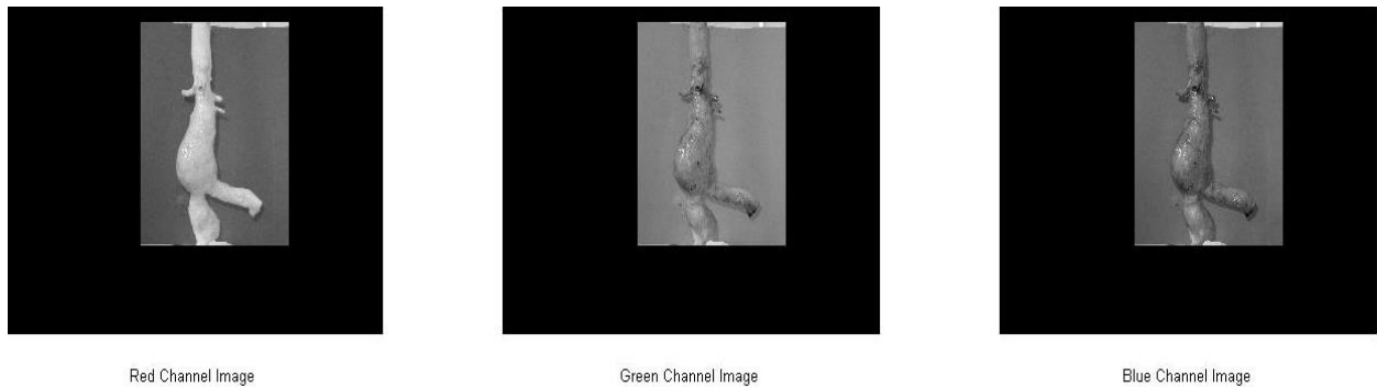
Figure 9: Decomposed image, red channel (left), green channel (center), and blue channel (right).
